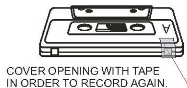
If later you do wish to record on side A of the cassette, cover the tab opening with a piece of cellophane tape. This will allow the Record ● to function again.
