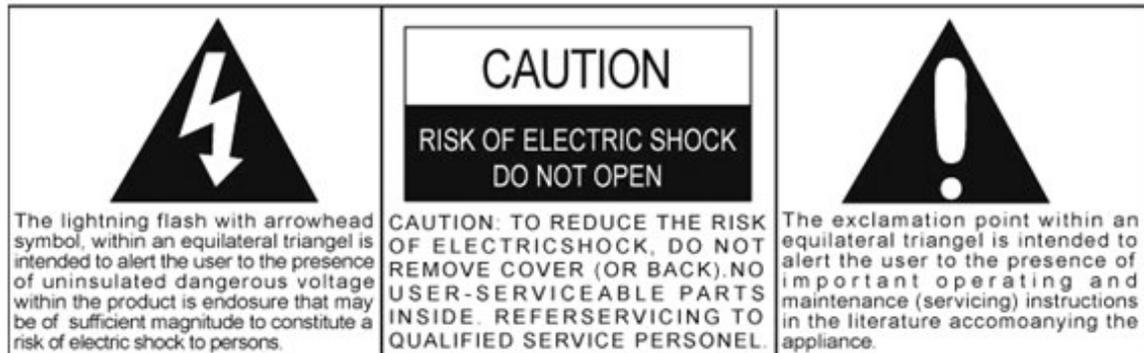
The Caution Marking is located at the bottom of the apparatus.
