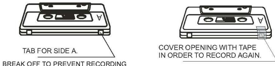
If later you do wish to record on side A of the cassette, cover the tab opening with a piece of cellophane tape. This will allow the Record ● to function again.
