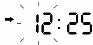
**Note:** The PM INDICATOR (#9) is located in the right part of the LED DISPLAY (#18). The PM INDICATOR (#19) will light when the hour digits selected are for PM time. The PM INDICATOR (#19) will be off when the hour digits selected are for AM time.
