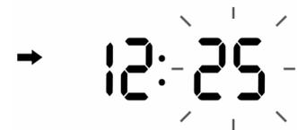
5. Tap the TIME BUTTON (#3) to confirm and complete the setting. The display will stop flashing.
