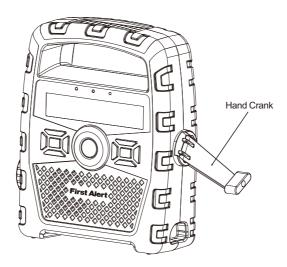
3.Continue turning the Crank to charge the internal battery. The longer you turn the hand crank, the more power you are generating to charge the battery, and the Radio listening time will be extended (Radio reception only).
