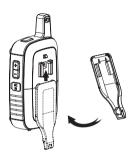
Carefully remove belt clip by sliding it downward to unlock it from its slot. Flip the belt clip over as shown below, and insert the small end of the belt clip into the locking tab as shown below. Once attached, the belt clip will becomes a stationary stand for use on a table top.
