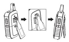
**Note**: To detach the stand, carefully push the stand downward. Do not pull the stand out and away from the unit, doing this may break the stand or the back of the cabinet and void the warranty.
