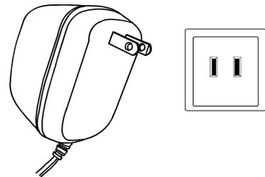
**CAUTION:** The system has an AC plug and will only fit into matching AC outlets. This is a safety feature to reduce the possibility of electric shock. If the plug will not fit in your AC outlets, you should have the outlet changed by a qualified, licensed electrician. Do not use an adaptor to make the plug fit into your outlet. This defeats the safety feature and could expose you to electric shock.
