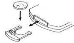
**IMPORTANT:** Be sure that the battery is installed correctly. Wrong polarity may damage the Remote Control and void the warranty.
