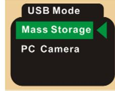
**Mass Storage:** After the camera connects with the computer in "Mass Storage" mode, then the LCD screen will be off and the BUSY light is on. "Removable Disk" in "My Computer" window will appear. The pictures or videos are saved in the Removable Disk. Choose the desired photo/video and copy (drag with mouse) it into the target folder of the computer.
